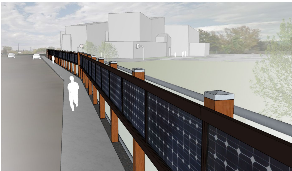
Figure 8-10. Fence Solar PV Options
